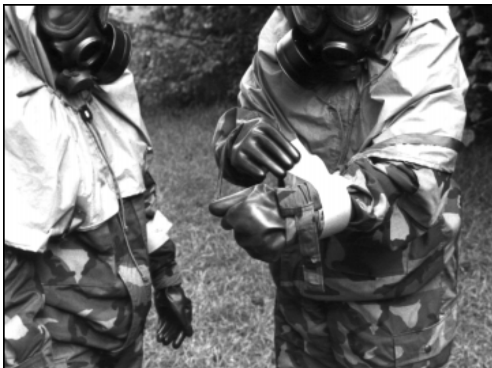
Figure 3-14. Putting on the M9 Detector Paper
